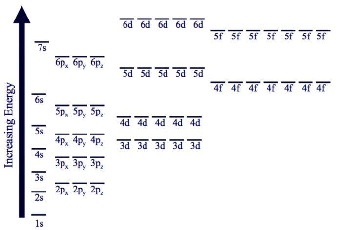
**HINT:** Use the periodic table to determine the number of electrons that are present in a krypton atom. An empty (no electrons) energy level diagram for multi-electron atoms is shown on the left. Electrons are arranged (configured) into the orbitals in the way that results in the lowest possible energy. Nature does this by obeying the Aufbau Principle, the Pauli Exclusion Principle, and Hund's Rules. See the hint from the previous question (3.2) for more details.
